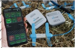
WiCow: vaginal temperature, calving detection, estrus detection
